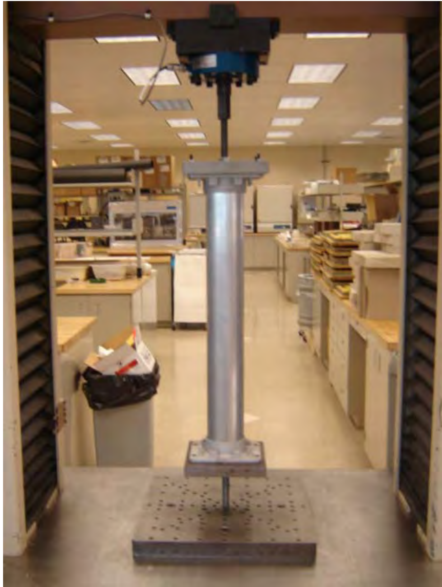
Photo No. 1 Uplift Resistance Test Setup
